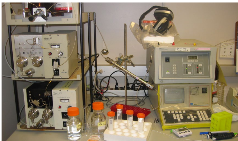
High-performance liquid chromatography was used to identify the molecular composition of cod liver oils.
